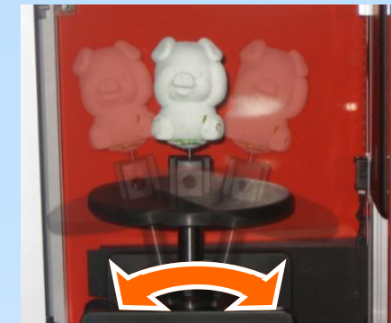
Adjustable Rotatory axis to turn different scan angle
