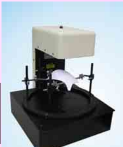
Utilize laser thickness measuring to compensate shrinkage & distortion
