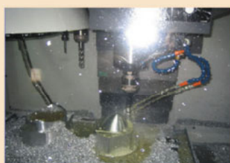
Produce master cone mould by CNC
