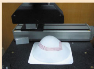
3D and texture high speed scanning for master cone
